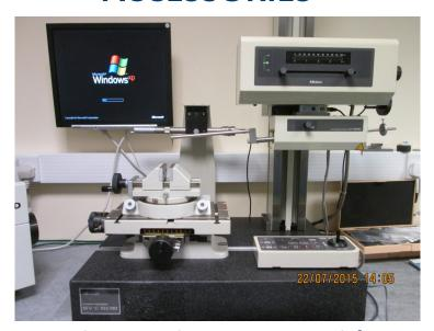
A high accuracy Mitutoyo instrument with accessories that allows measurement of surface roughness and form/contour.
